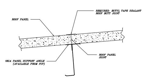
\*NOTE:USE FIELD APPLIED SPRAY FOAM AS NEEDED TO MAINTAIN VAPOR BARRIER AND INSULATION CONTINUITY
