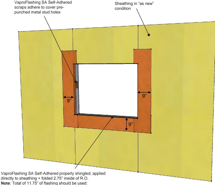
9" of flashing should be left on the face of the sheathing
