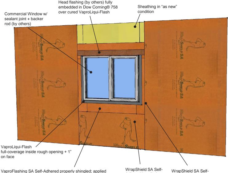
directly to sheathing + folded 2.75" inside of R.O. Note: Total of 11.75" of flashing should be used:
