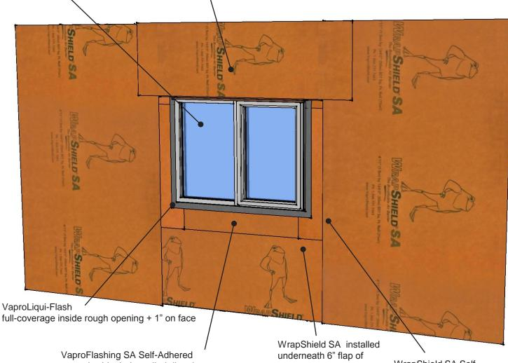
properly shingled; applied directly to sheathing + folded 2.75" inside of R.O. VaproFlashing SA to create shingle effect
