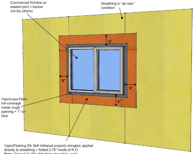
Note: Total of 11.75" of flashing should be used:
