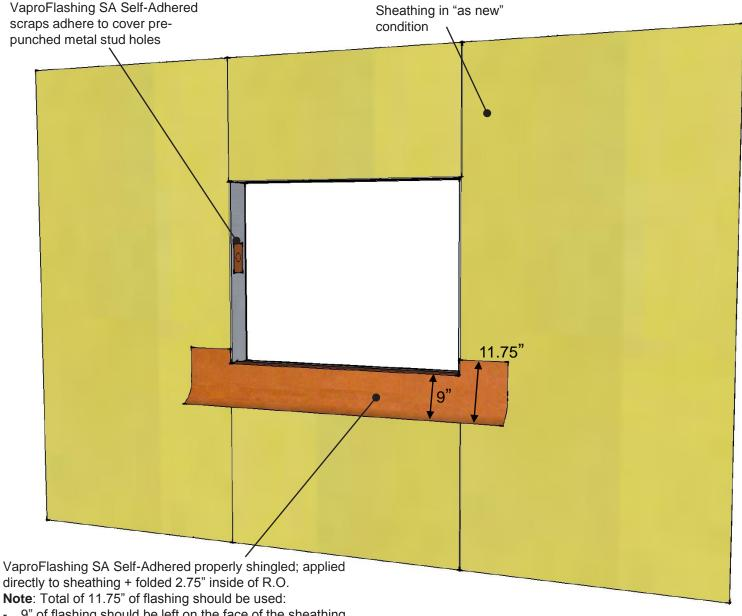
9" of flashing should be left on the face of the sheathing
